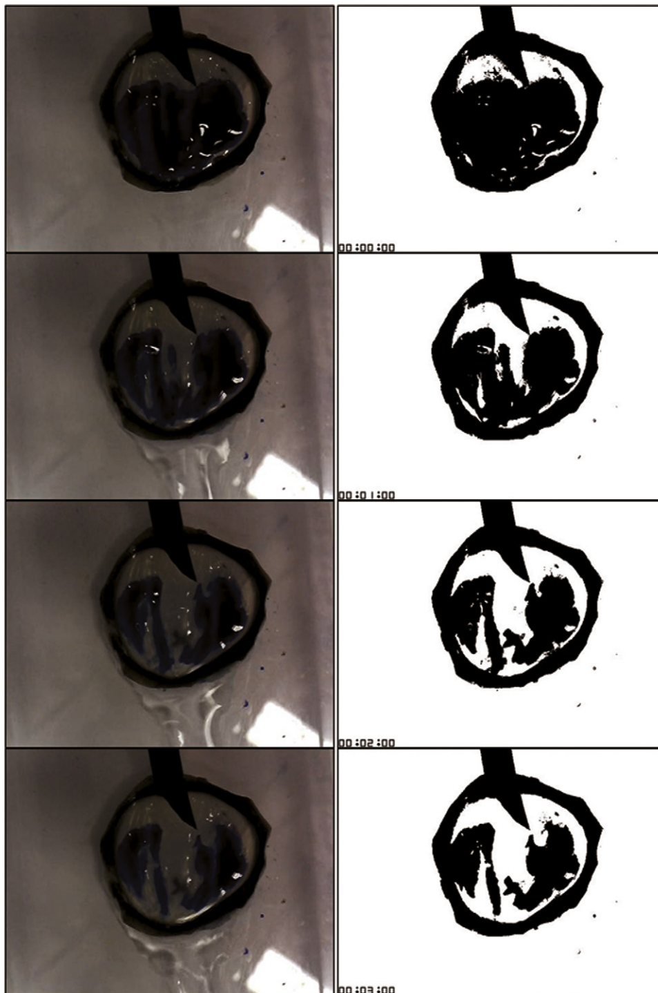
Fig. 4. A comparison of images of gelled Carbopol 971 PNF neutralized with 4% (v/v) of 0.5 M NaOH before (left) and after (right) thresholding.
